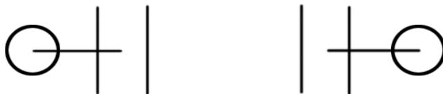
There is a small circle that is shifted away from the center of each pair of vertical lines by a distance that is proportional to and in the direction of the stick displacement (shown above for left stick pushed forward.) Each small circle is connected by a line to the center of the pair of vertical lines.
